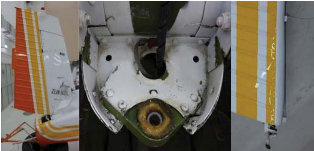
Figure 14 - Rudder and Vertical Stabiliser Deformation
