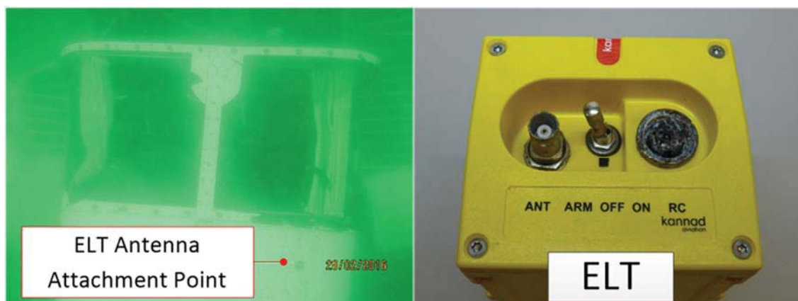
Figure 18 - ELT Location and ARM Switch
