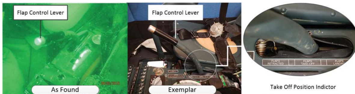
Figure 9 – (Left) Flaps control lever as found underwater. (Right) exemplar for reference
